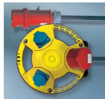
1 CEE socket 16A, 5P, 400V 2 SCHUKO® sockets 16A, 230V with 3m of supply cable H07RN- F5G2.5 with CEE plug 16A, 5P, 400V Ref. no. 94356
